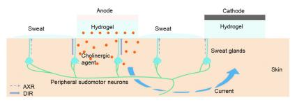
Figure 14. Scheme of iontophoresis-based sweat induction. AXR: Axon-reflex mediated sweating. DIR: direct stimulated sweating.
