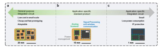
Figure 29. Strategies for choosing which types of integrated circuits to use for designing a wearable electronic device.  $\mathbf{a} - \mathbf{c}$ , Electronic components can be categorized based on degree of integration as general purpose integrated circuits (GPICs) (a), application specific standard products (ASSPs) (b), and application specific integrated circuits (ASICs) (c).
