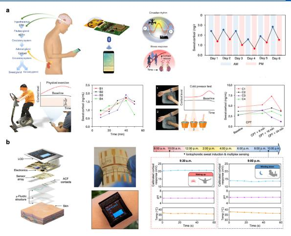
Figure 35. Wearable sensors for stress monitoring. a, A fully integrated, flexible, and wireless mHealth device, for stress response monitoring in sweat cortisol. Reproduced with permission from ref 93. Copyright 2020 Elsevier. b, A wearable aptamer-field-effect transistor-based smartwatch with signal correction algorithm for sweat cortisol detection. Reproduced with permission from ref 91. Copyright 2022 The American Association for the Advancement of Science.
