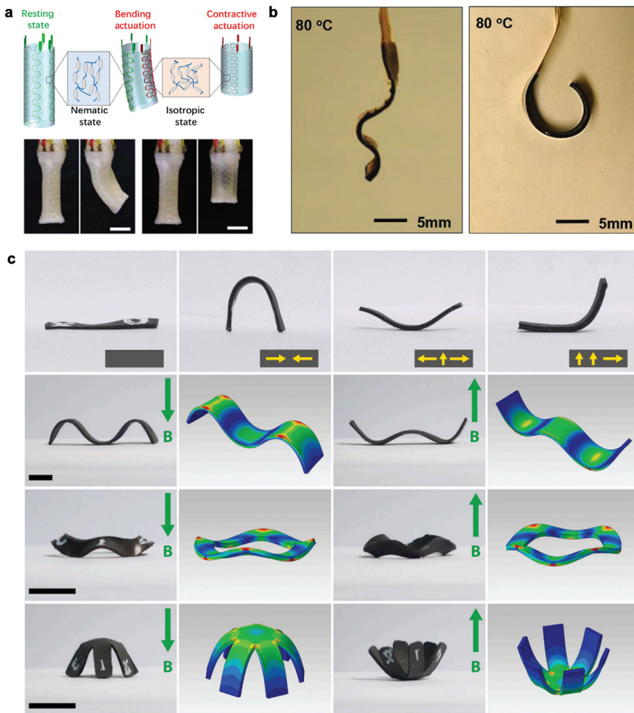
Figure 4. Multimodal actuators that are responsive to a single stimulus. a) By selectively applying electrical potential, the tubular actuator made of liquid crystal elastomer demonstrates both bending and uniform contraction modes. b) Utilizing a carbon black-doped liquid crystal elastomer nanocomposite, complex shape manipulation is achieved, resulting in diverse actuation motions through the strategic placement of Kapton film in different positions. c) Through the combination of hard magnetic particles and stretchable silicone rubber, a reconfigurable actuator exhibited a range of magnetization patterns and undergoes multimodal shape transformations when subjected to a magnetic field. a) Reproduced with permission. [139] Copyright 2019, AAAS. b) Reproduced with permission. [107] Copyright 2018, John Wiley & Sons. c) Reproduced with permission. [141] Copyright 2021, Elsevier.
